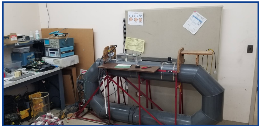
Recirculating Flow Loop
